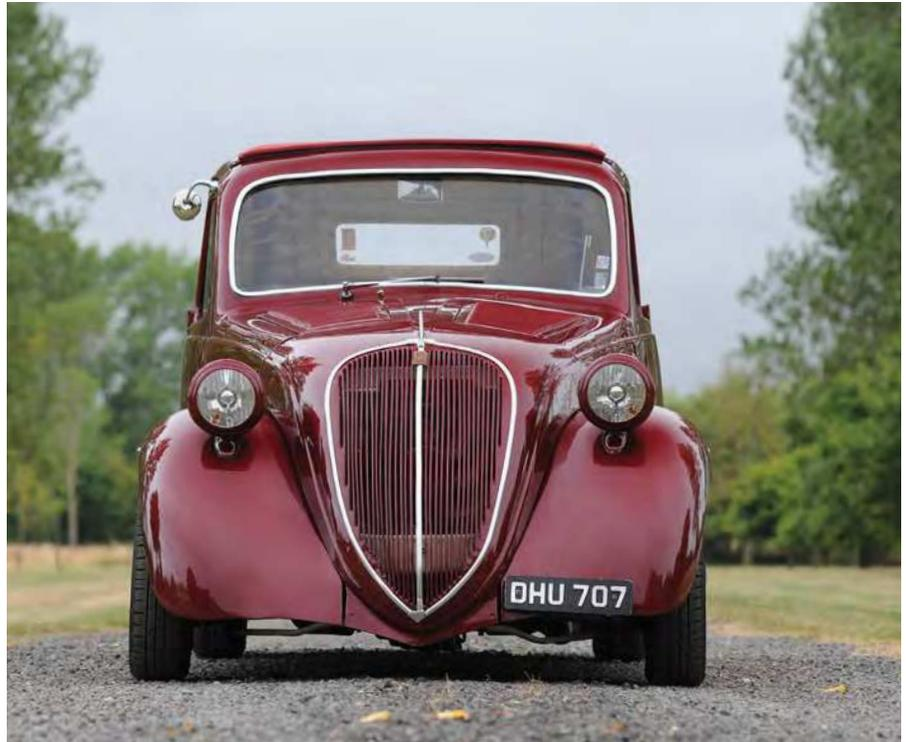
crashing over the slightest bump. That's because the engine sits very low, with a notably low-hanging exhaust (it exits under the sill because there's no room for it to be routed to the back), so the stiff set-up is needed to avoid bottoming out.
